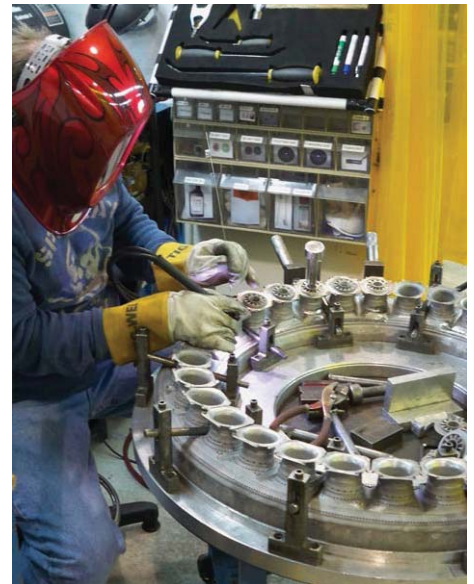
Weld repair process on a CF6-50 combustor dome Jet Aviation Specialists
